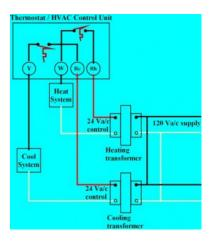
The next step up from the older home systems was the introduction of the 'fan on / auto' switch. This function allows you to circulate the air in the house by using the fan in the furnace without heating or cooling the air moving through the system.
